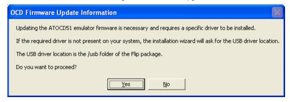
2. Then Select "Yes", the "batchisp" program is launched in a command window and fails : the command window exits and the green system LED of OCD system stops blinking.
